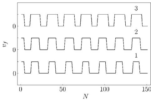
FIG. 2. Periodic regions of capture and transmission as a function of the number  $N$  of defects with  $d=0.2$  for different initial velocities  $v_0$ . The lower horizontal parts (with  $v_f=0$ ) correspond to capture and the upper ones (with  $v_f>0$ ) to transmission. Curves 1, 2, and 3 correspond to  $v_0=0.048, 0.050,$  and  $0.052,$  respectively.
